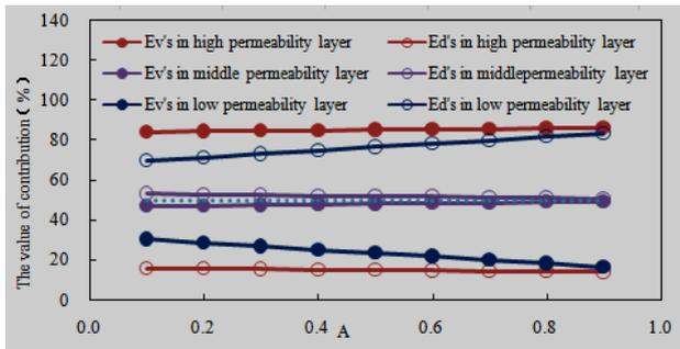
Fig.3 The contribution of each layer at polymer flooding stage for two-dimensional heterogeneous physical model
