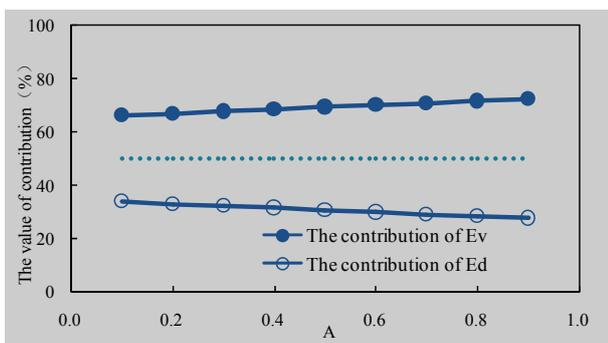
Fig.4 The contribution at binary combination flooding stage for two-dimensional heterogeneous physical model
