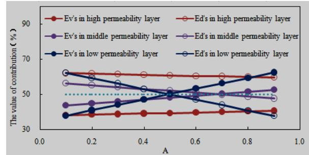
Fig.5 The contribution of each layer at binary combination flooding stage for two-dimensional heterogeneous physical model
