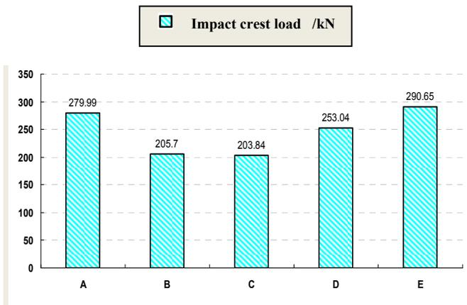
Figure14. The five pipes impact crest value
