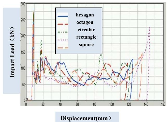
Figure8. Displacement - impact load curves.
