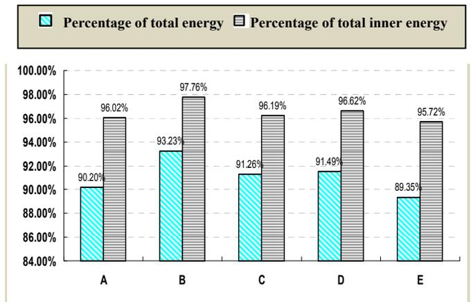
Figure12. The five pipes absorbing energy percentage
