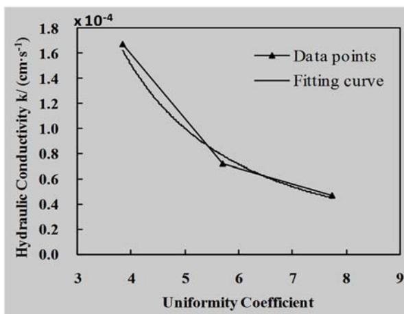
Fig 10. Relationship between slag hydraulic conductivity and  $C_u$
