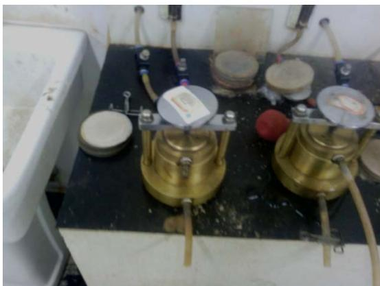
Fig 4. The apparatus of South 55-type variable head permeameter.
