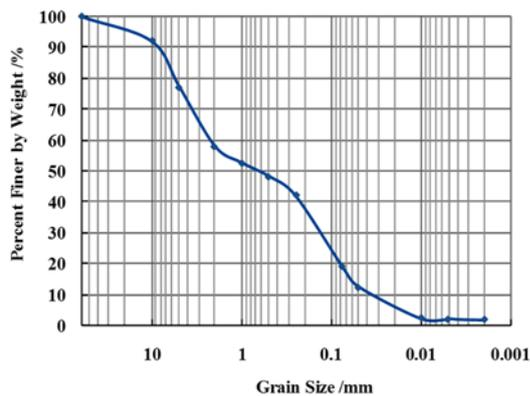
Fig 1. Grading curve of original slag.
