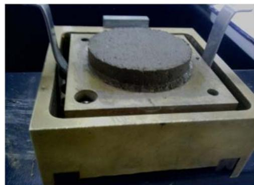
Fig 3. The direct shear apparatus and broken samples.
