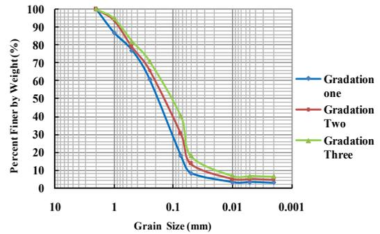
Fig 2. Grading curves of three remodeling samples.
