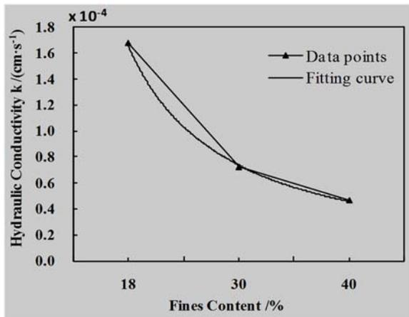
Fig(9). Relationship between hydraulic conductivity and fine particles content of slag samples.
