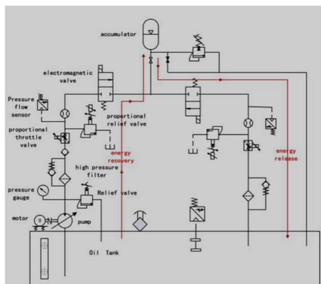
Fig1. Working Principle Map of Vehicles Regenerative Braking Simulation System
