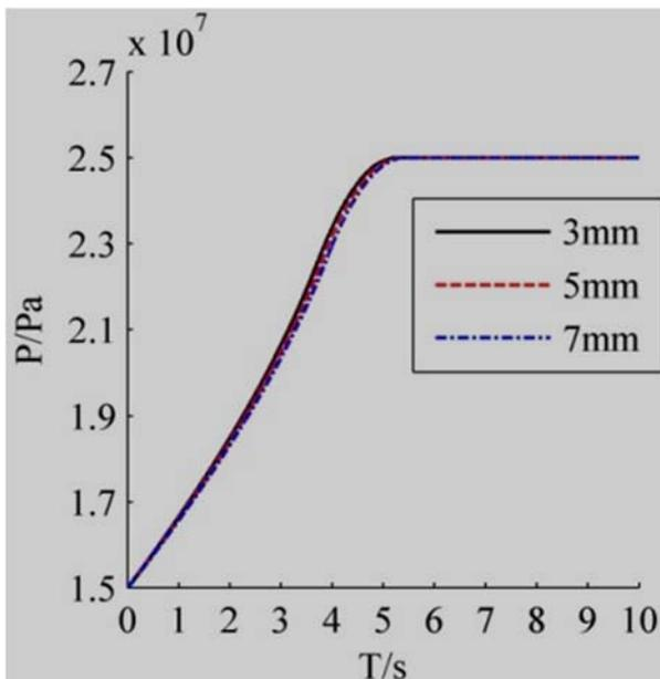
Fig4. The Pressure Change Curve of Different Pre-compression of Spring.
