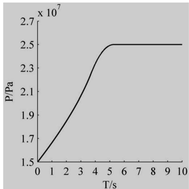
Fig2. The Pressure Change Curve of the Regenerative Accumulator
