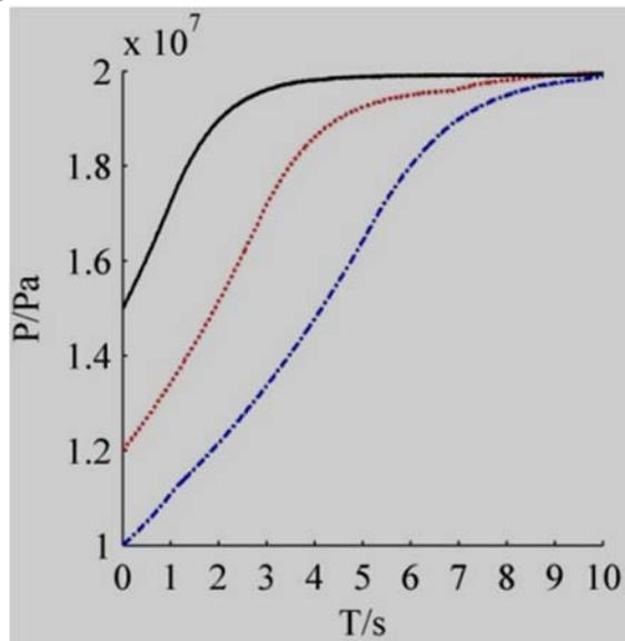
Fig6. Changing curves of pressure under three different initial low pressures.
