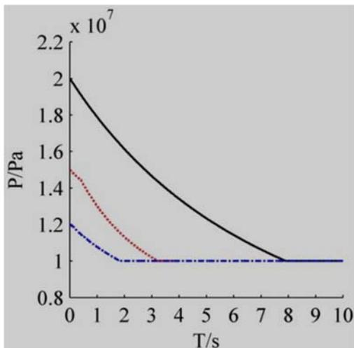
Fig7.Changing curves of pressure under-three different initial high pressures
