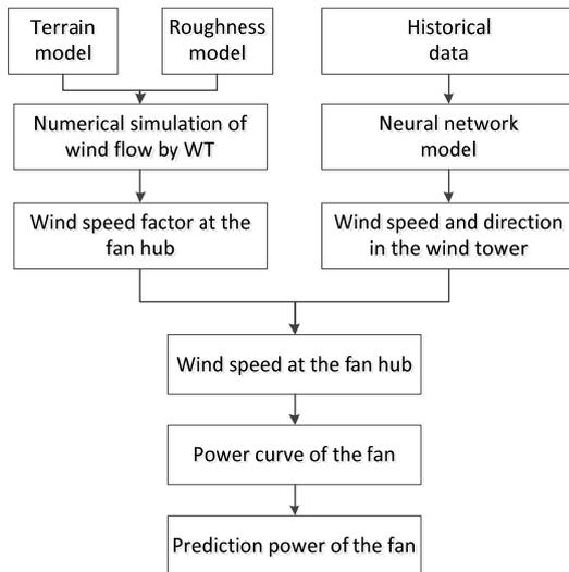
Fig. (1).flow chart of the wind power prediction
