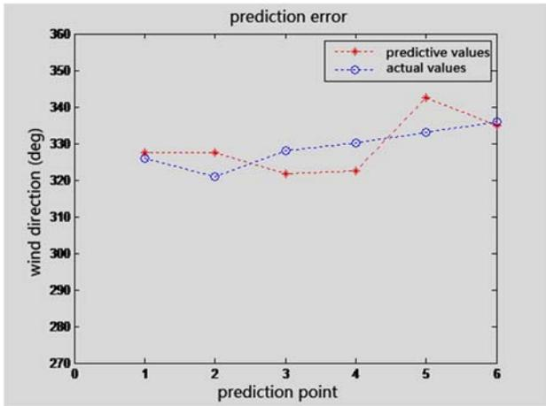
Fig. (3).Comparison between actual and predictive value of wind direction.
