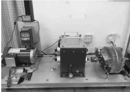
Figure 2. Subway gearbox test bench
