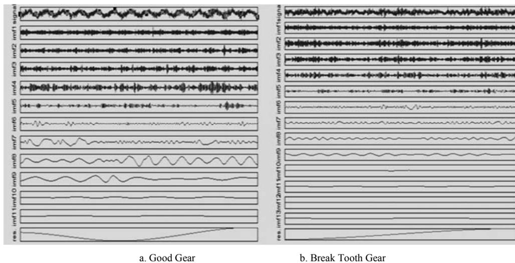
Figure 3. IMF of Gear Signal
