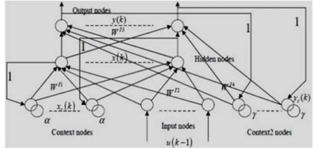
Figure 1. Schematic Diagram of OHF Elman Neural Network
