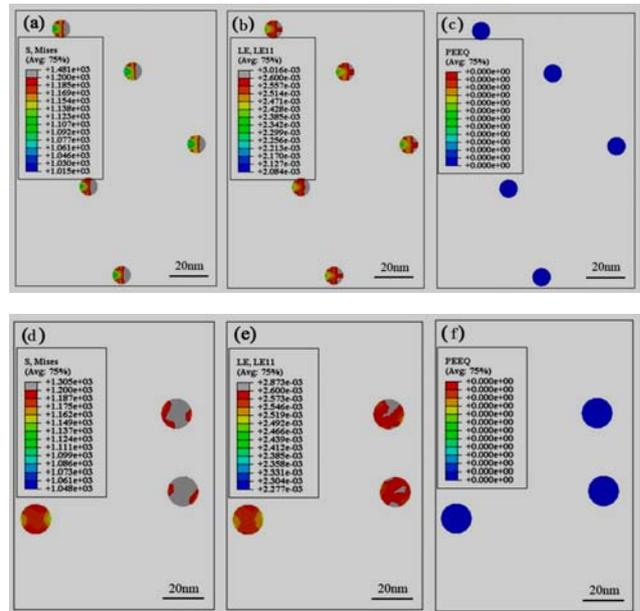
Fig.7. The Contours of Equivalent Stress, The Strain Component LE11 and The Equivalent Plastic of Strain in Difference Size of VC Precipitates: (a), (b), (c), 10nm; (d), (e), (f) 20nm.
