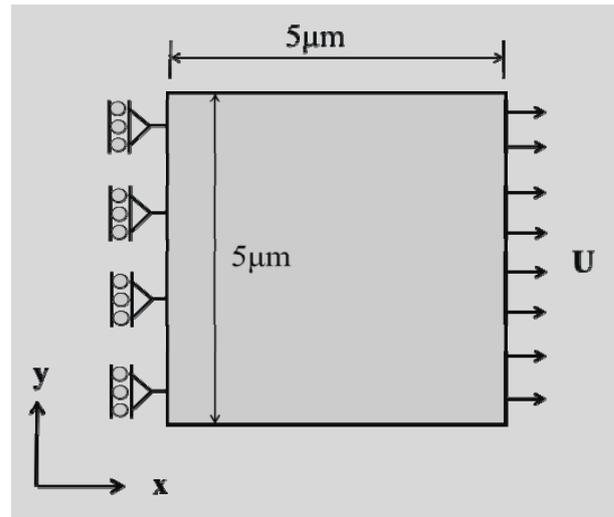
Fig.2. Example of boundary conditions and loads.
