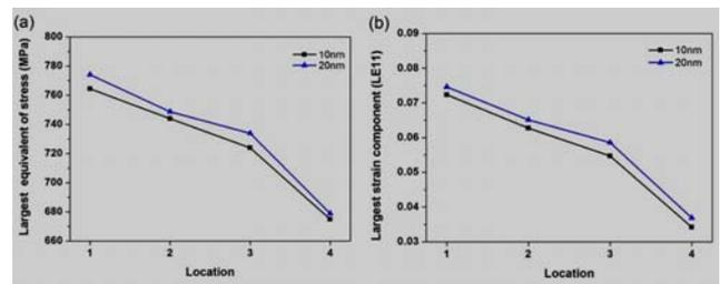
Fig.5. Variation of the largest equivalent stress and the largest strain component LE11 of matrix at the location with different sizes of VC precipitates
