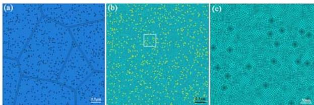
Fig.1. Finite element model of VC precipitates: (a) no meshing model, (b) meshing model, (c) enlarged view
