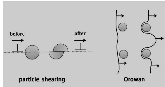
Fig.9. The contours of equivalent stress in “folded back” (A to B) region for different sizes of VC precipitates: (a) 10nm; (b) 15nm; (c) 20nm; (d) dislocation movement mechanism
