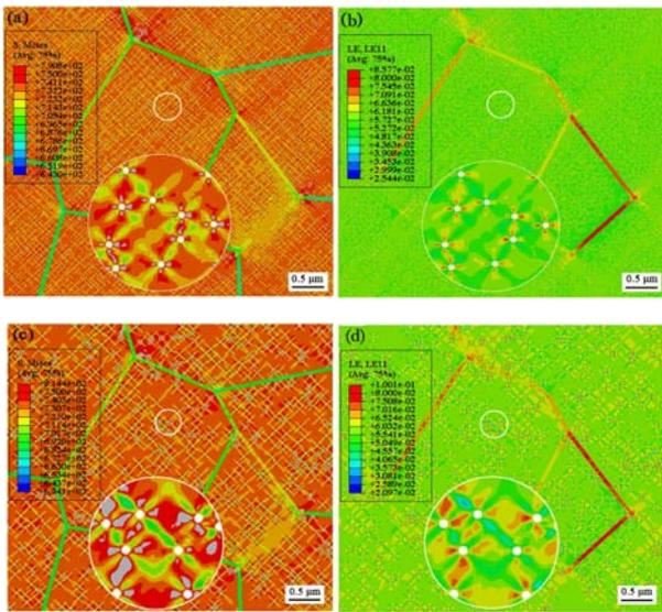
Fig.6. Contours of VC precipitates of equivalent stress and strain component LE11 in matrix: (a) (b) 10 nm; (c) (d) 20 nm
