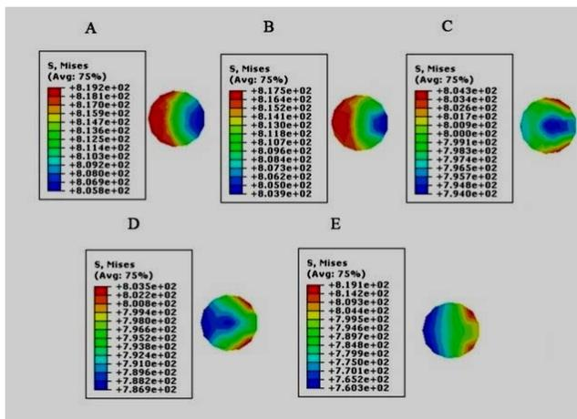
Fig.8.The contours of equivalent stress in “folded back” (A to B) region for different sizes of VC precipitates 10nm
