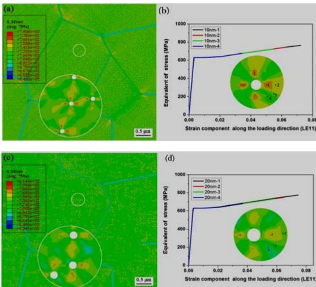
Fig.4. Contours of equivalent stress in the matrix and stress-strain curve in different place: (a) (b) 10 nm; (c) (d) 20 nm
