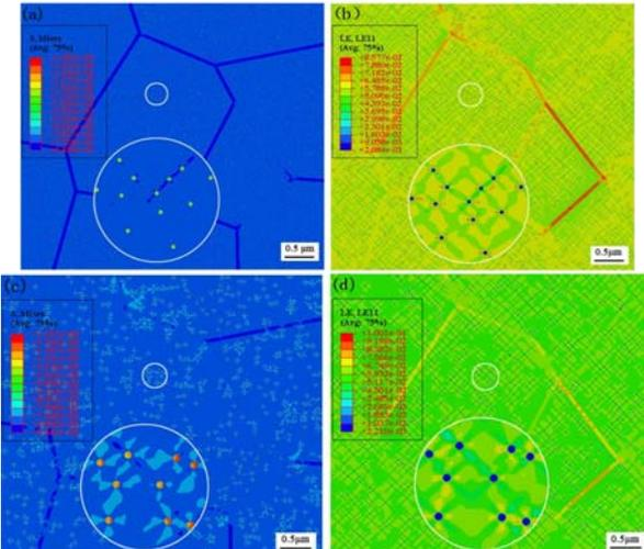
Fig.3 Contours of the equivalent stress and the strain component LE11 of VC precipitates: (a) (b) 10nm; (c) (d) 20nm
