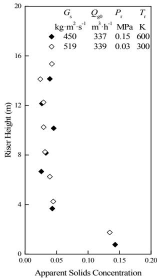
Figure 3. Axial profile of apparent solids concentration of different particles under different temperature and pressure.
