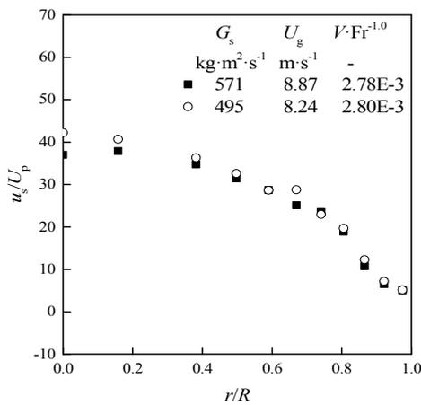
Figure 4. Radial profile of dimensionless solids velocity of Sand II.
