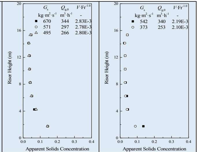
Figure 2. Axial profile of apparent solids concentration of Sand II
