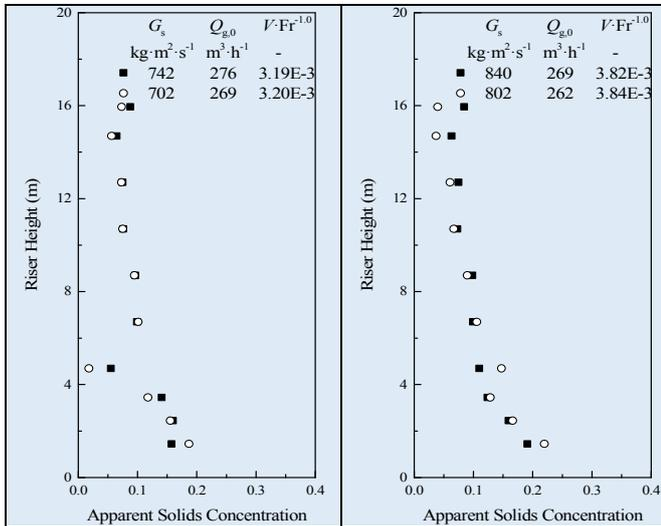
Figure 1. Axial profile of apparent solids concentration of Sand I
