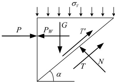
Figure 3. Forces acting upon the wedge with water pressure
