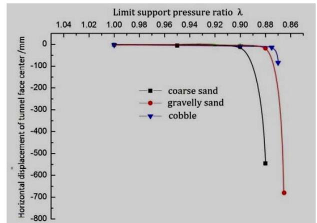
Figure 7 Horizontal displacement of the central point of tunnel face
