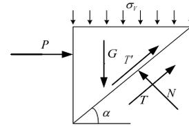
Figure 2. Forces acting upon the wedge without water pressure
