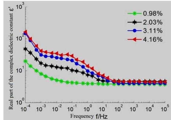
Fig.4 Real part of the complex dielectric constant at different moisture contents at 25°C
