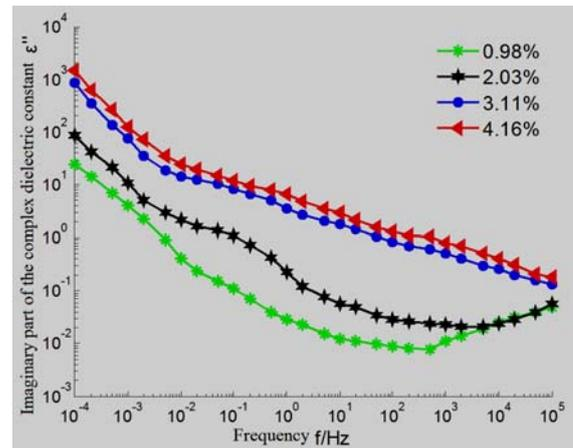
Fig.5 Imaginary part of the complex dielectric constant at different moisture contents at 25°C
