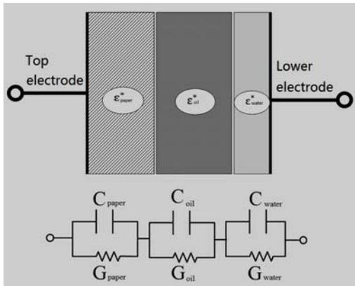
Fig.3 The equivalent three-phase insulation system model of oil, paper and water.
