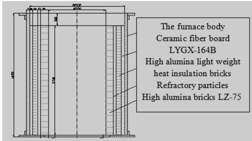
Fig. 2 The Structure of Furnace Body after Optimization
