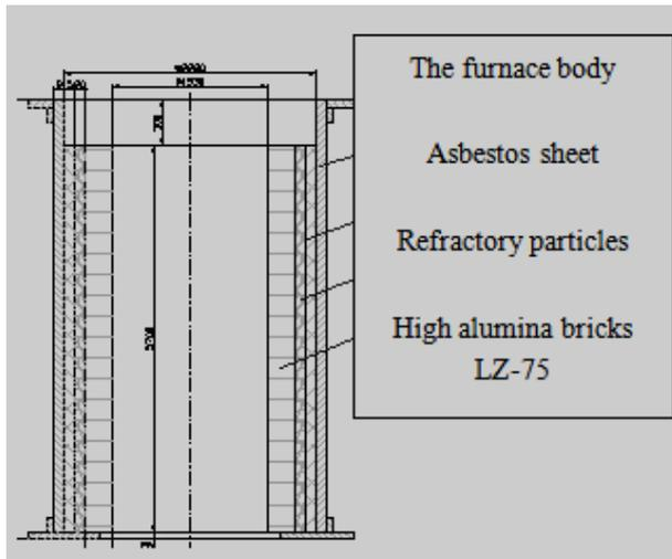
Fig. 1-B. The Existing Electric Calcined Furnace and Structure of Furnace Body
