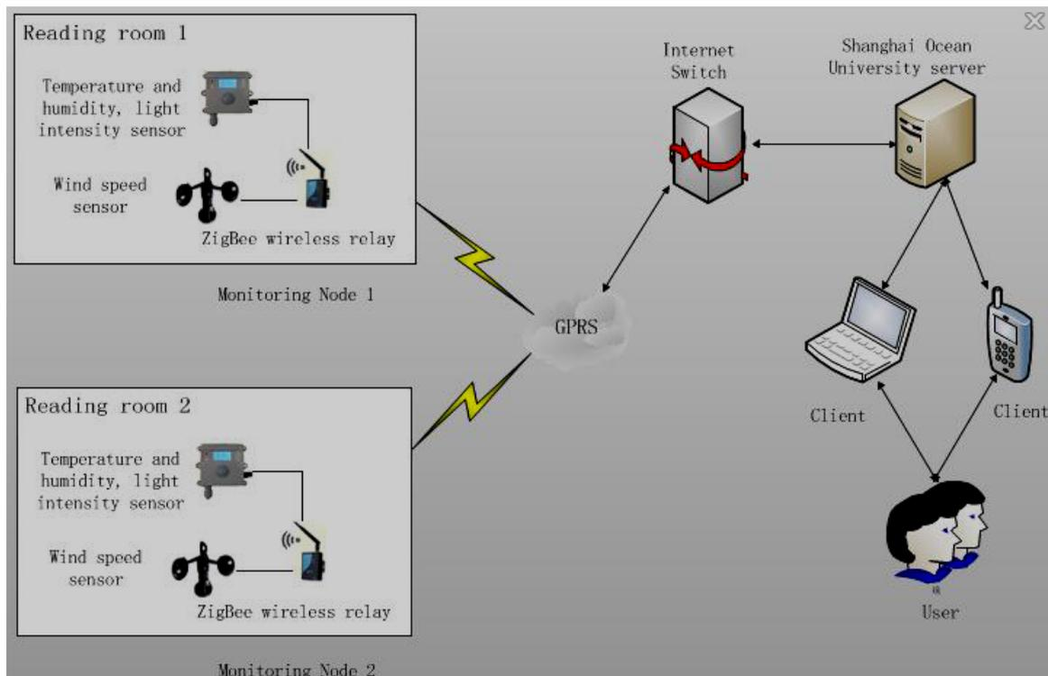
Fig2. The structure of library environment monitoring system
