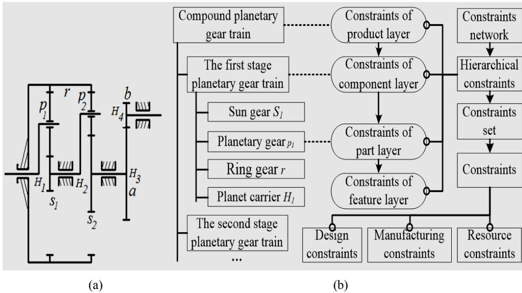
Fig. 1 Transmission diagram of compound planetary gear train and its constraints.
