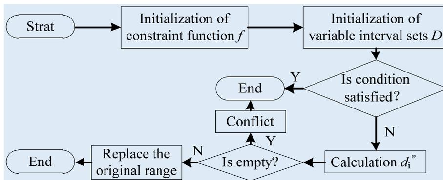
Fig. 3 Detection process based on interval propagation algorithm.
