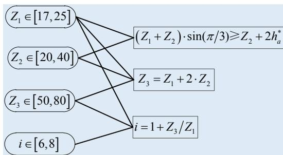
Fig. 4 Constraint network of adjacent planetary gear trains without Noise.
