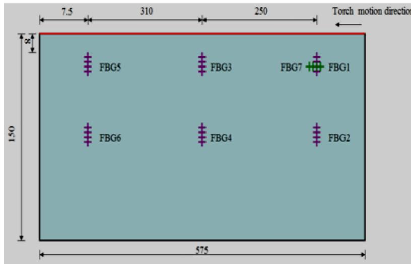
Fig.3. FBGs Layout in the welding stress measurement of the aluminum alloy plate
