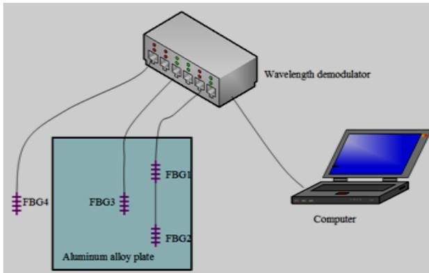
Fig.1 FBG arrangement in temperature and stress calibration experiment.
