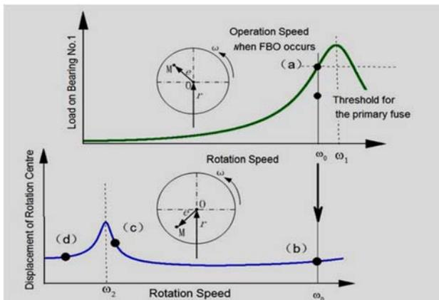
Figure 2. Scheme of the mechanisms of LRD
