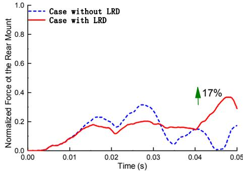
Figure 15. Radial reaction force of the rear mount
