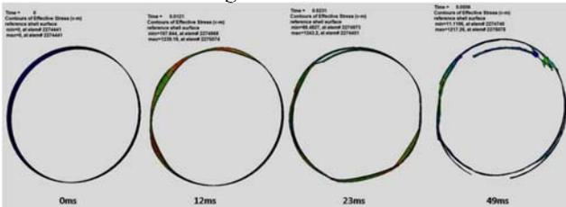
Figure 8. Progressive failure of the hollow cone for the case with LRD
