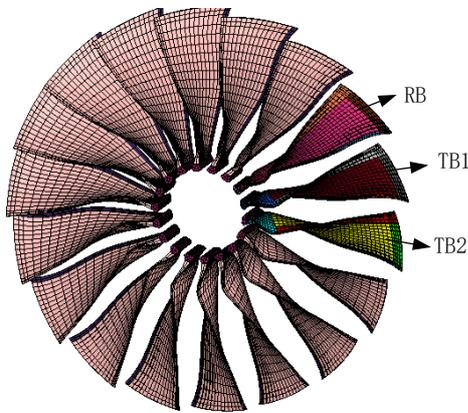
Figure 4. Finite Element Model of the Fan Blades
