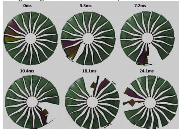
Figure 5. Progressive damage of fan blades for case with LRD
