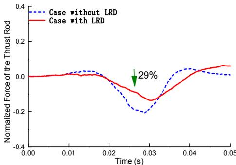
Figure 16. Axial reaction force of the thrust rod
