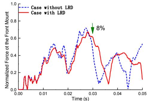
Figure 14. Radial reaction force of the front mount
