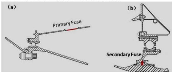
Figure 1. Scheme of the load reduction device: (a) thin section; (b) fuse pin
