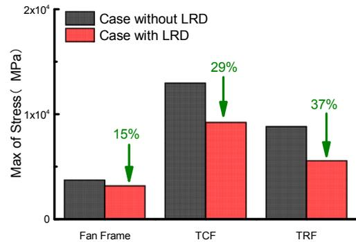
Figure 17. Maximum equivalent stress of main load-bearing frames
