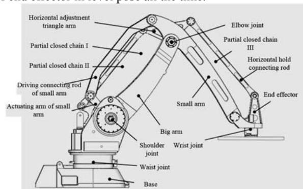
Figure 1. Structure diagram of MD-1200YJ stacking robot
