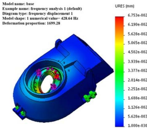
Figure 6. Cloud picture of base displacement
