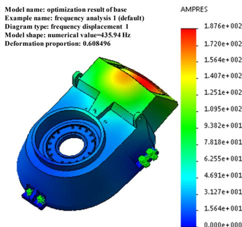
Figure 14. Vibration mode diagram of first order after optimization
