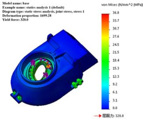
Figure 5. Cloud picture of base stress
