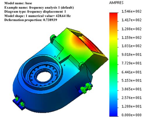
Figure 7. Vibration mode diagram of first order of base
