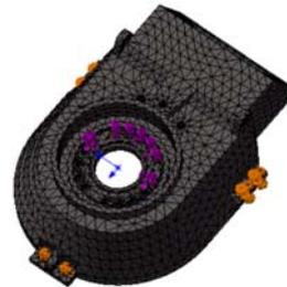
Figure 4. The finite element model of base
