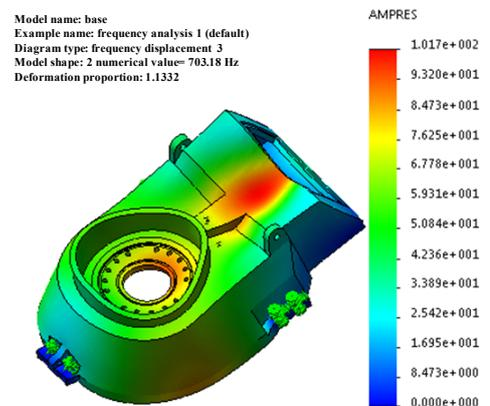
Figure 9. Vibration mode diagram of third order of base
