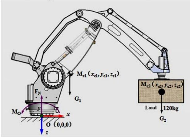
Figure 2. Stress analysis of moving part
