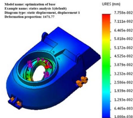
Figure 16. Displacement diagram after optimization
