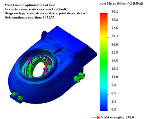
Figure 15. Stress diagram after optimization
