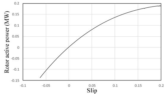
Figure 6. Active power absorbed by rotor under changes of slip
