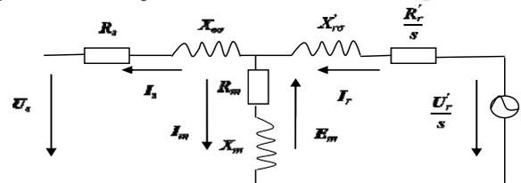
Figure 2. DFIG equivalent circuit
