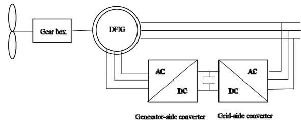
Figure 1. The structure diagram of doubly-fed wind power generator
