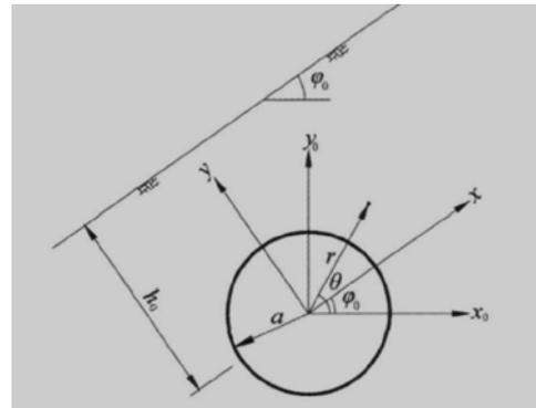
Figure 1. Stress analysis of bias tunnel
