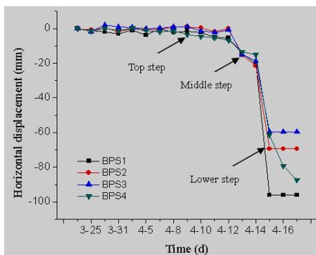
Figure 9. The relationship between horizontal displacement and tunnel excavation (DK15+010)
