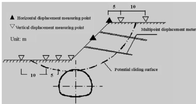
Figure 4. Slope displacement measuring plan
