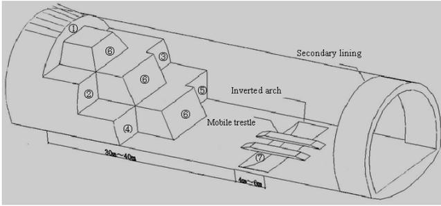
Figure 3. Excavation process of bias tunnel
