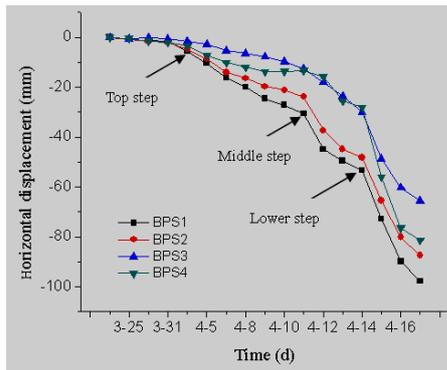
Figure 8. The relationship between horizontal displacement and tunnel excavation (DK15+000)
