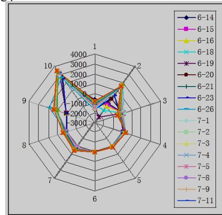
Figure 6. Bending moment distribution of steel support
