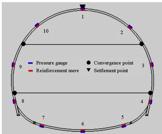
Figure 5. Stress and displacement measuring of tunnel surrounding rock
