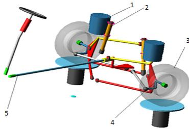
1. Air spring assembly 2. Shock 3. Tire 4. Steering knuckle connecting bracket 5. Steering assembly
