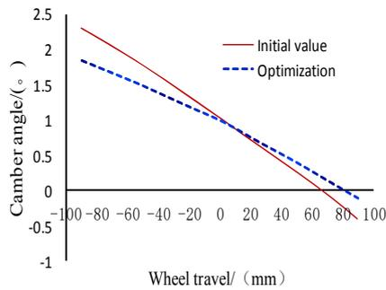
Fig. 7 Comparison of camber angle
