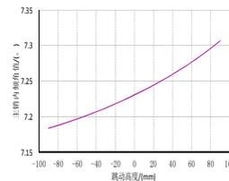
Fig.4 Change curve of kingpin inclination angle
