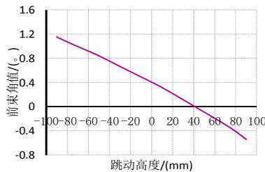
Fig.2 Change curve of toe angle with the wheel
