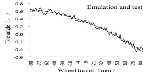
Fig. 13 Test validation of toe angle
