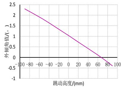
Fig.3 Change curve of camber angle
