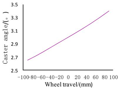
Fig. 5 Change curve of caster angle
