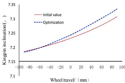
Fig.9 Comparison of kingpin inclination angle
