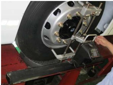
Fig.11 Front wheel clamps and probe
