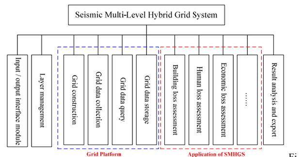
Figure 3 Functional structure of SMHGS
