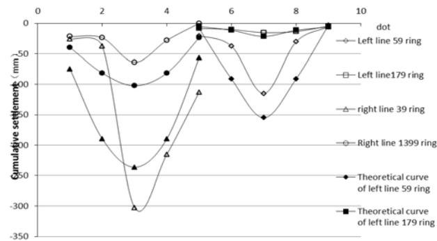
Figure6. Theoretical and measured comparison chart of cross-sectional
