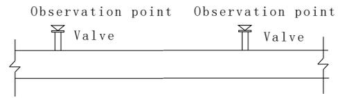
Figure5. schematic diagram of underground pipe line subsidence monitoring
