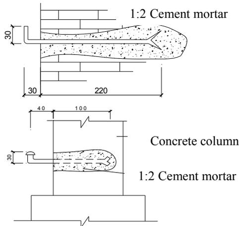
Figure4. Schematic diagram of the surrounding buildings embedding measuring points (unit: mm)
