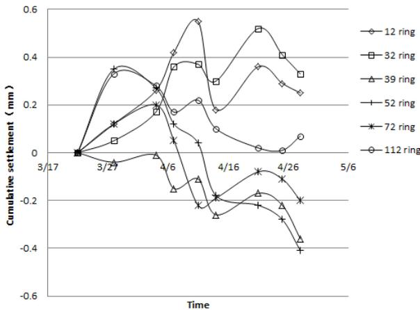
Figure9.The left line vault settlement last graph
