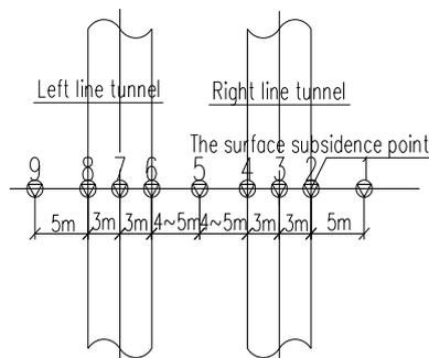
Figure 1. Surface Monitoring Section Points
