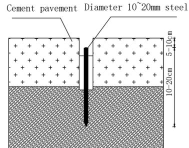
Figure 3. schematic diagram of embedding ground settlement point
