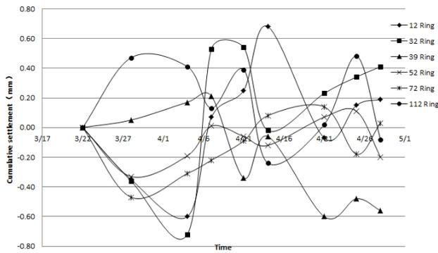
Figure8. The left line arch bottom settlement last graph
