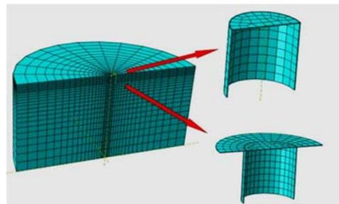
Figure 1. Finite element model
