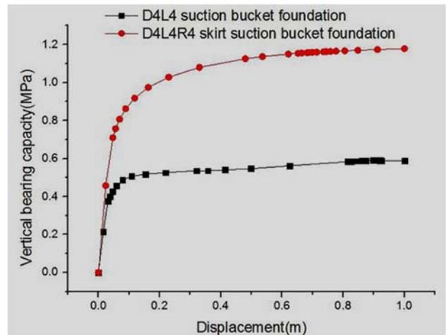
Figure 3. Vertical bearing capacity of different foundation
