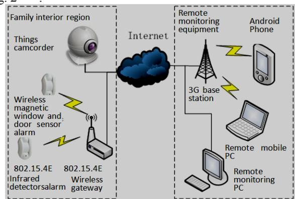
Fig. 2 The Diagram of System Network
