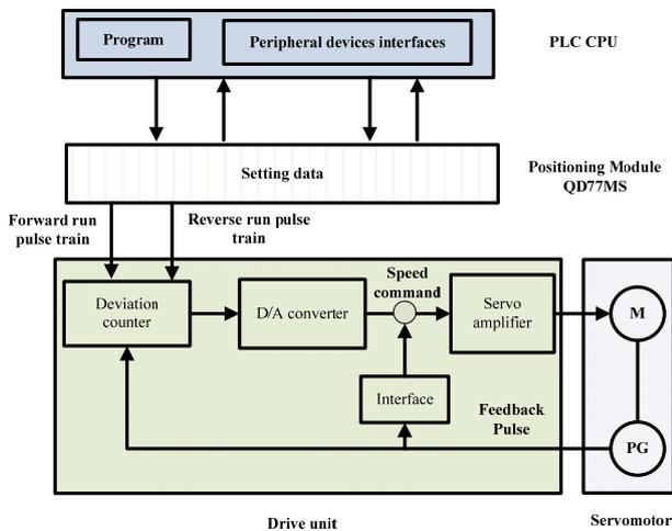
Figure 4. Outline of the positioning operation of QD77MS
