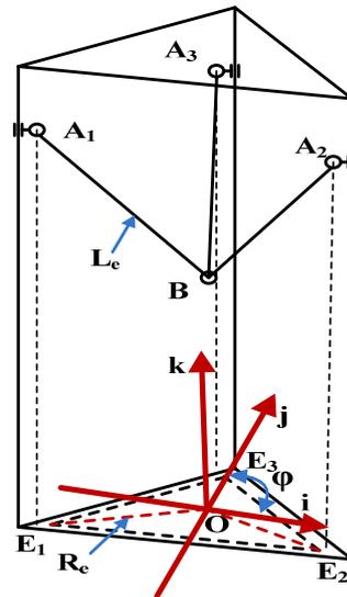
Figure 6. A visual representation of inverse kinematics
