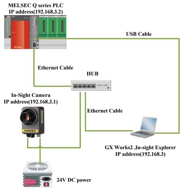
Figure 5. Connection configuration for the vision system
