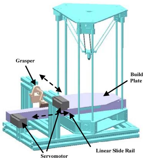
Figure 2. Specific view of movable build plate and grasper
