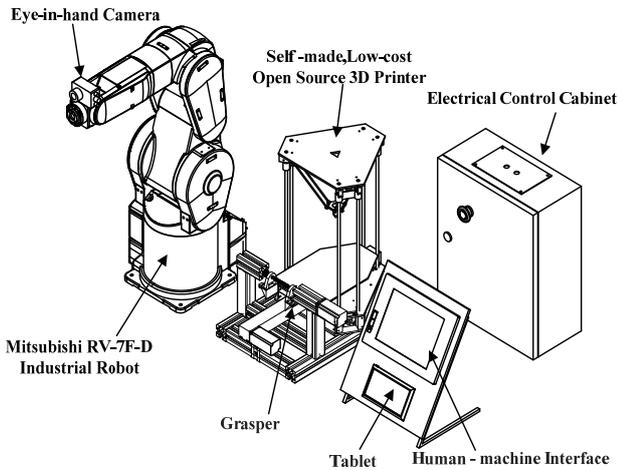
Figure 1. System configuration
