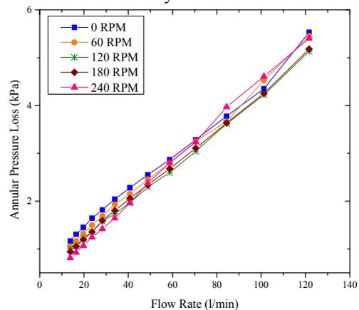
Figure 5. Annular pressure loss with flow rate for different rotation speeds
