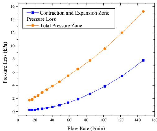
Figure 7. Tool-joint total and contraction and expansion zone pressure losses with flow rate
