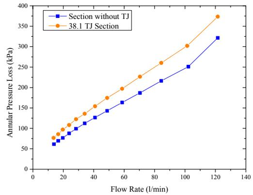
Figure 4. Comparison of annular pressure loss for one stand of drillpipe with one joint at different flow rates
