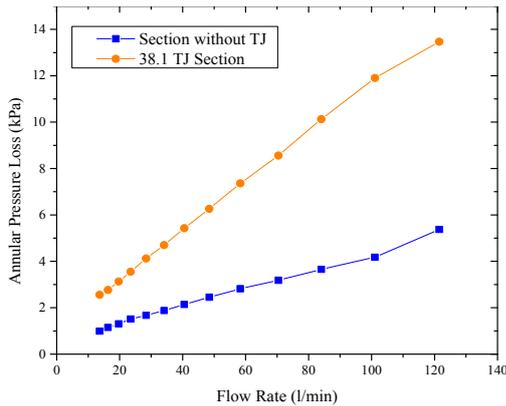
Figure 2. Comparison of annular pressure loss with and without tool-joint for different flow rates
