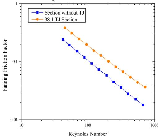
Figure 3. Comparison of fanning friction factor with and without tool-joint for different Reynolds numbers
