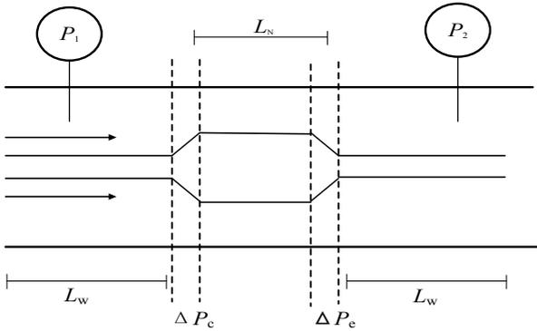
Figure 1. Schematic of tool-joint
