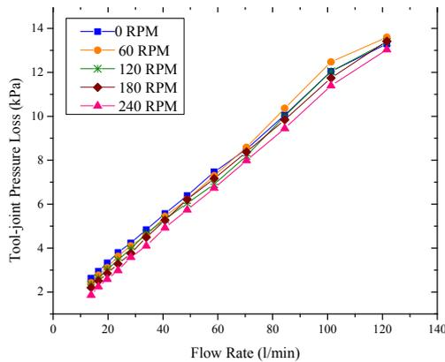
Figure 6. Tool-joint pressure loss with flow rate for different rotation speeds
