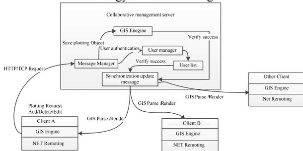
Figure.2 Logical Process of Collaboration Technology
