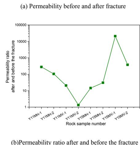
Figure 13. Permeability after and before the mudstone fracture
