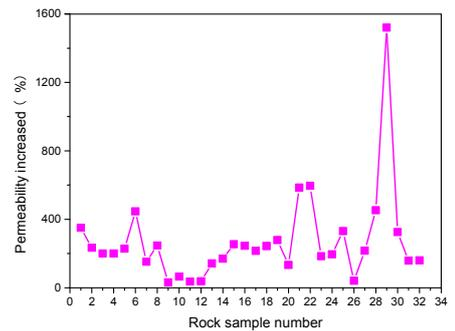
Figure 7. Sandstone permeability increase with decreased pressure
