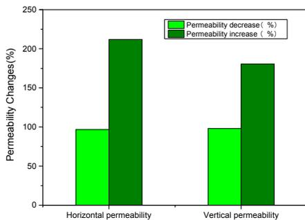
Figure 11. Comparison of average horizontal and vertical permeability
