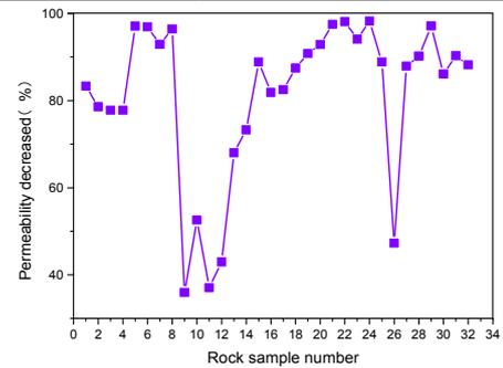
Figure 6. Sandstone permeability decrease with increased pressure
