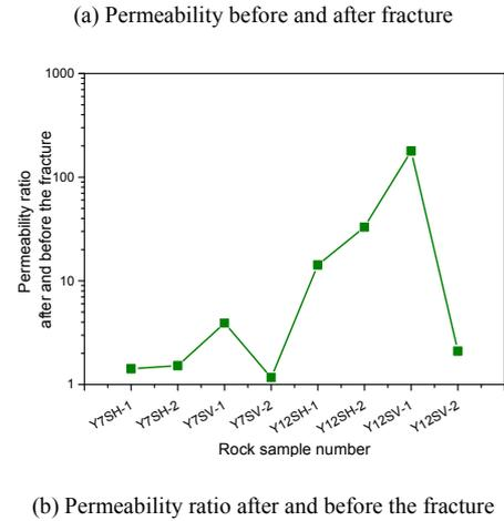
Figure 12. Permeability after and before the sandstone fracture
