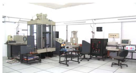
Figure 3. Triaxial rock mechanics testing system
