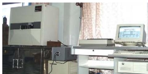
Figure 2. CMS series core auto analyzers
