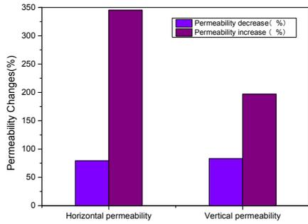
Figure 8. Comparison of average horizontal and vertical permeability of sandstone samples
