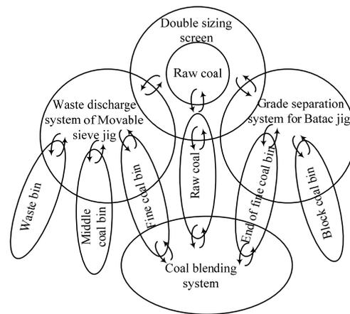
Figure 2. CPS model of coal preparation plant
