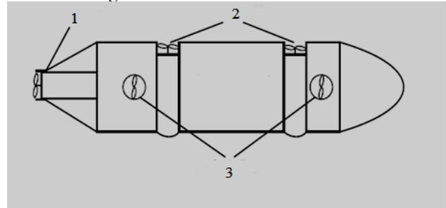
1- the main propulsion, 2-the lifting propulsion, 3-the steering propulsion
