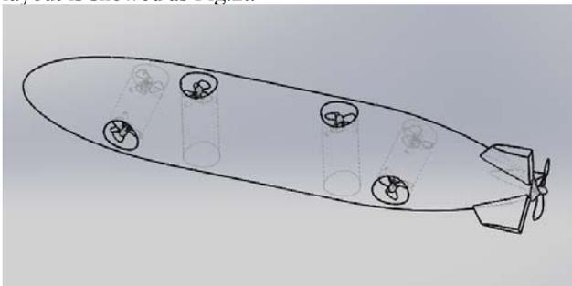
Figure 2. The specific layout of the propulsion
