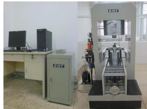
Figure 1. RMT-301 rock and concrete mechanics test system
