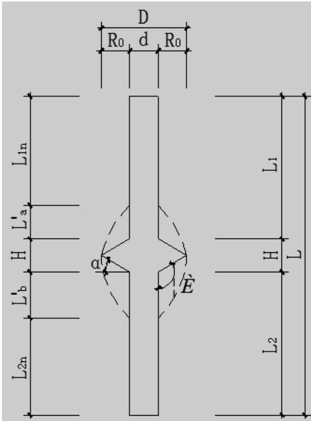
Figure 1. The diagram of pile under vertical tension
