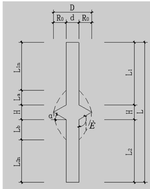
Figure 2. The diagram of pile under vertical compression
