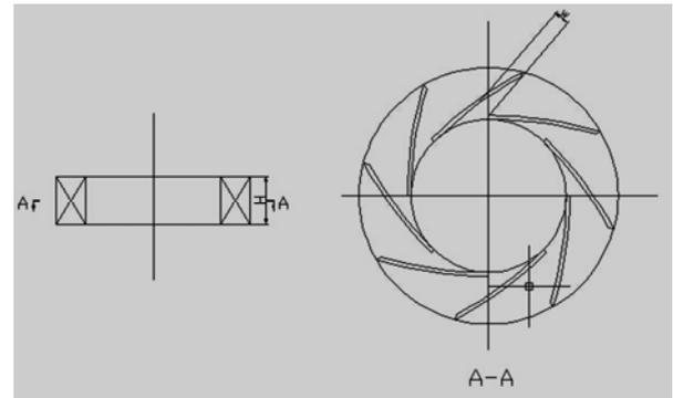
Figure 2. Structural diagram of the swirl generator.
