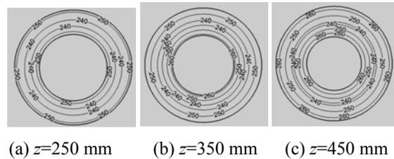
Figure 9. The isolines of  $T$  at different position of the nozzle separation section (K).
