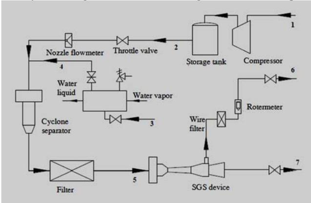
Figure 4. Schematic diagram of the experimental process of SGS device.
