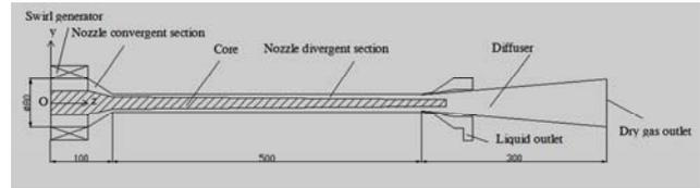
Figure 1. Structural diagram of the SGS device.
