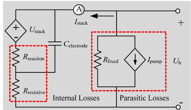
Figure 2. Equivalent circuit model of VRB.
