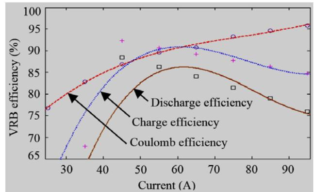
Figure 7. Simulation waveforms of VRB efficiency.
