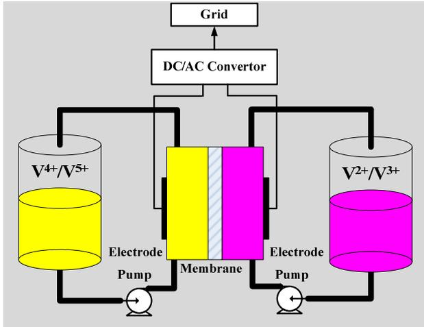
Figure 1. VRB operating principle.
