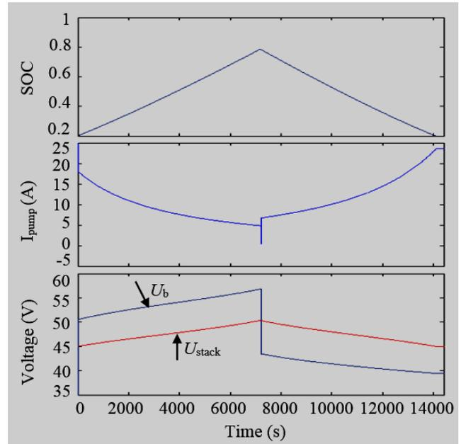
Figure 3. Simulation waveforms of VRB charge-discharge.
