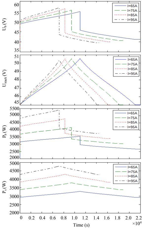
Figure 4. Simulation waveforms under constant current mode.
