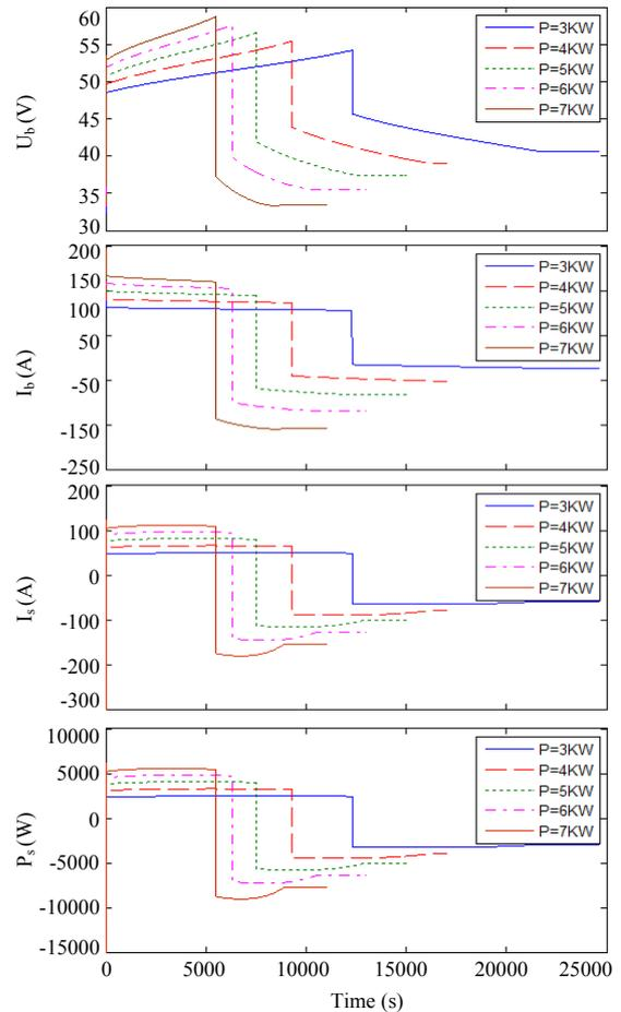
Figure 5. Simulation waveforms under constant power mode.
