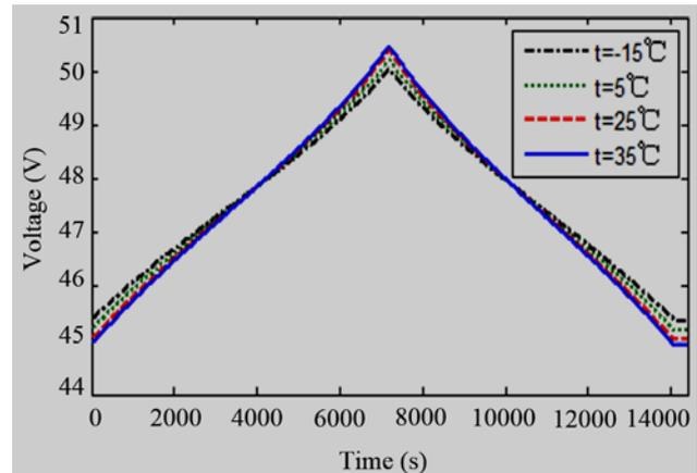
Figure 9. VRB stack voltage at different temperature.
