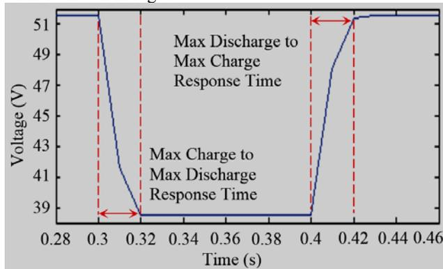
Figure 8. Transient characteristic of VRB.
