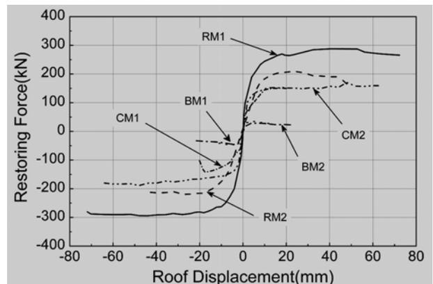
Figure9. Skeleton curves obtained from experiment
