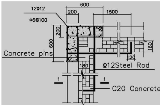
Figure 3. Joints: wall-to-concrete-columns
