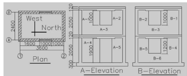
Figure 1. Plan view and elevation of building (dimensions in mm)
