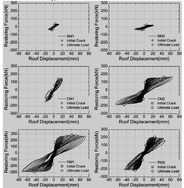
Figure.8. Hysteretic curves during low cyclic tests.
