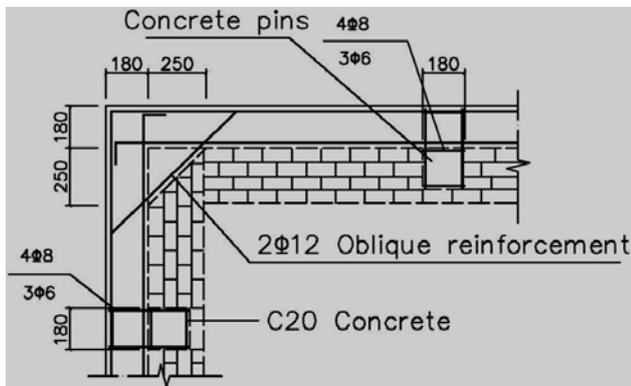
Figure 4. Joints: (wall-to-concrete-beams)
