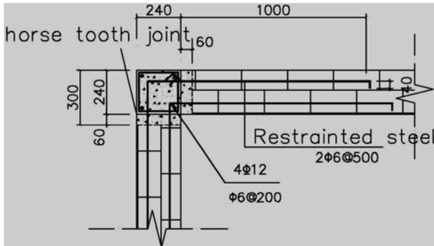
Figure 2. Joints: wall-to-tie-columns
