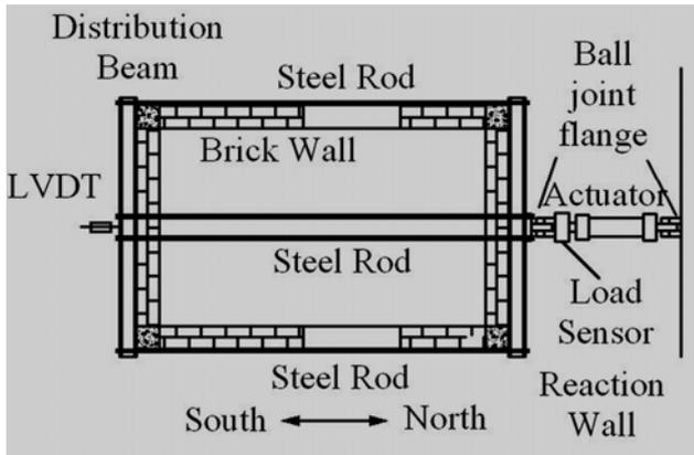
Figure 7. Plan view of Test loading system.
