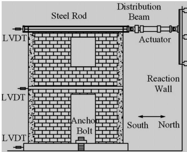
Figure 6.. Elevation view of Test loading system
