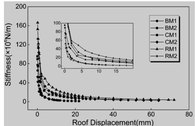
Figure10. Stiffness degradation curve of models.
