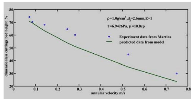
Fig.9 The influence of flow rate for dimensionless cuttings bed height comparison predicted data with martins' experimental data.
