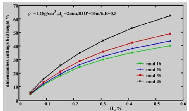
Fig.6 The influence of cuttings volumetric concentration for dimensionless cuttings bed height
