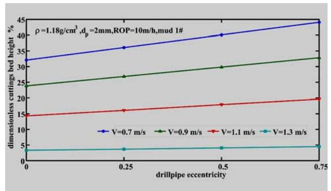
Fig.5 The influence of drill-pipe eccentricity for dimensionless cuttings bed height
