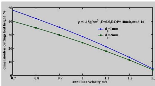
Fig.7 The influence of flow rate for dimensionless cuttings bed height with different cuttings diameter
