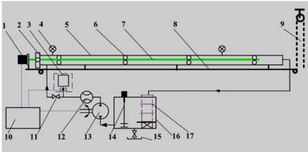
Fig.1 Schematic diagram of experimental apparatus for horizontal slim hole.
