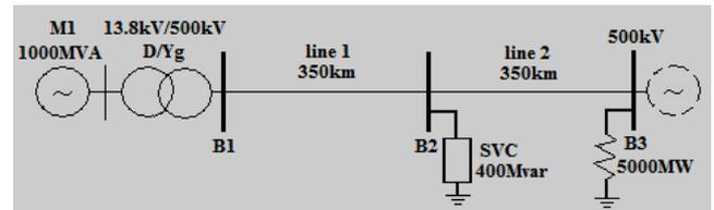
Fig.1 A Single Line Diagram of SMIB with SVC
