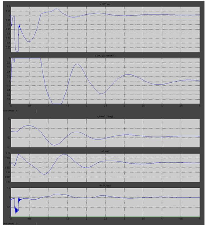
Fig.4 Impact of the SVC for a Three-Phase Fault (Fault applied at t=0.1 s and cleared at t=0.2 s).
