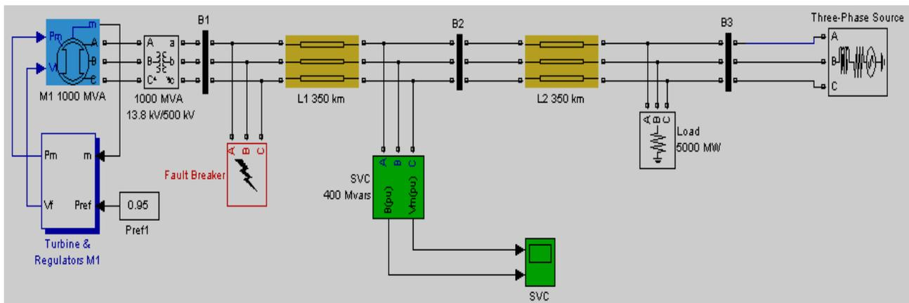
Fig.2 Simulation Model of SMIB with SVC
