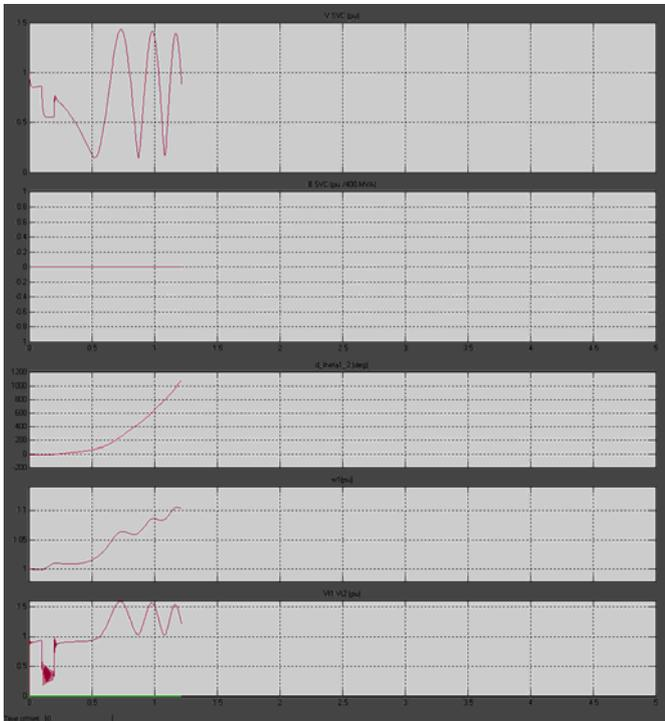
Fig.3 Impact without SVC for a Three-Phase Fault (Fault applied at t=0.1 s and cleared at t=0.2 s)
