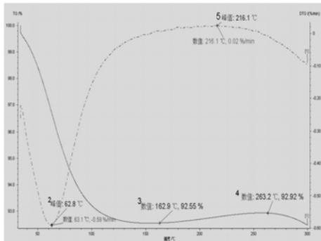
Figure (h) TGAcurve chart (oxygen concentration 13%)
