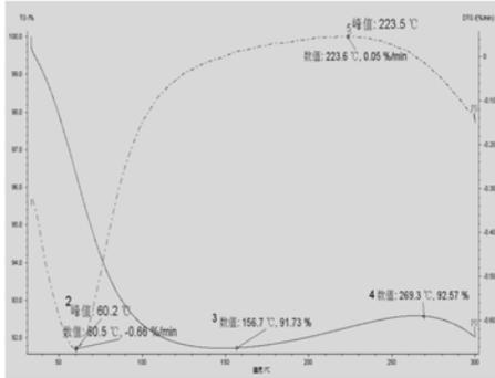
Figure (e) TGAcurve chart (oxygen concentration 21%)
