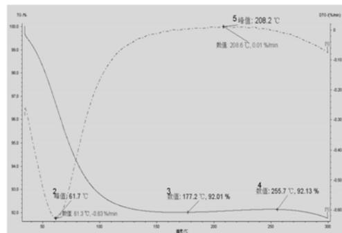
Figure (k) TGAcurve chart (oxygen concentration 7%)
