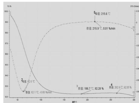
Figure (j) TGAcurve chart (oxygen concentration 9%)
