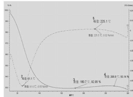
Figure (i) TGAcurve chart (oxygen concentration 11%)
