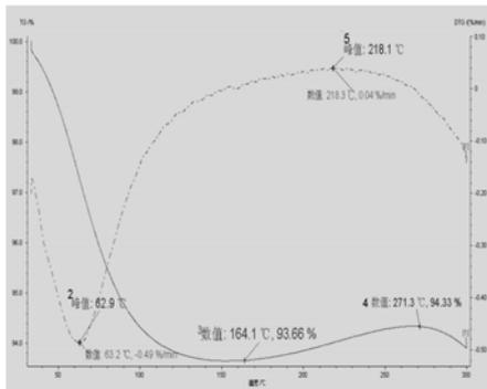
Figure (f) TGAcurve chart (oxygen concentration 18%)
