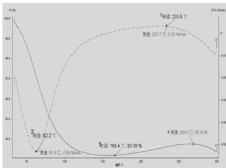
Figure (g) TGAcurve chart (oxygen concentration 15%)
