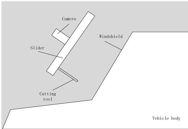
Figure 1. Framework of windshield cutting system.
