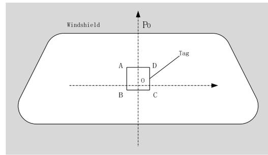
Figure 2. Principle of image process for windshield profile.
