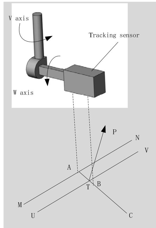
Figure 5. Tracking method for trajectory planning.
