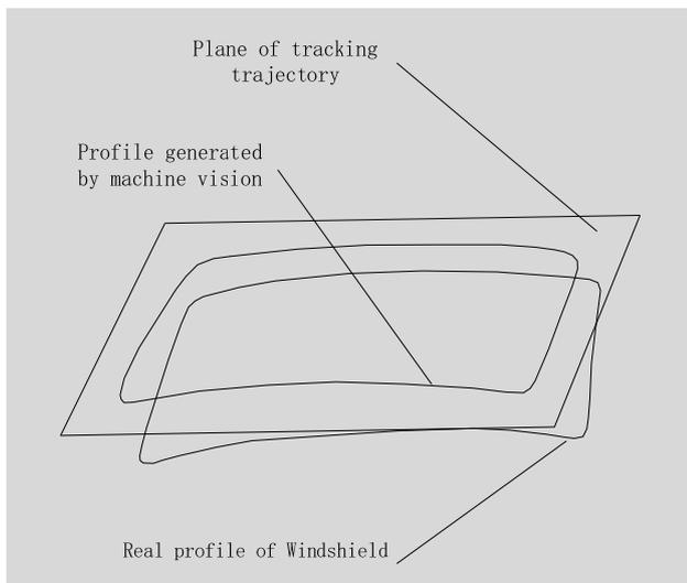
Figure 4. 2D profile of and the 3D profile of windshield.
