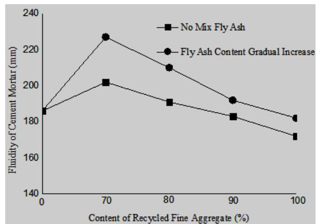
Figure1. Recycled Fine Aggregate Influence on Cement Mortar Fluidity
