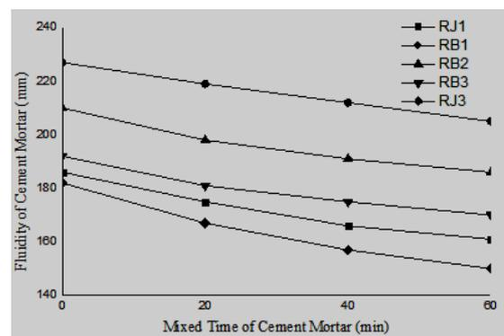
Figure3. Recycled Fine Aggregate and Fly Ash Effect of Compound Admixture on Cement Mortar Fluidity Loss
