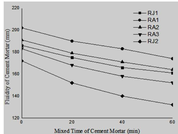
Figure2. Recycled Fine Aggregate Influence on Cement Mortar Fluidity Loss
