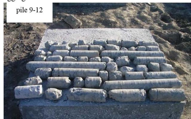
Figure 5. Pre-drilling embedded geotextile gravel grouting pile drilling core.
