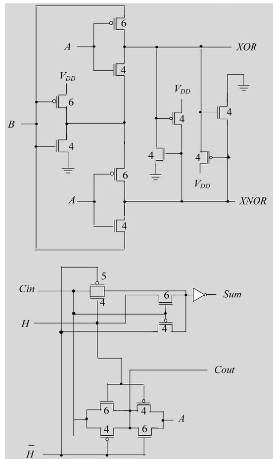
Figure 9. The proposed full swing hybrid full adder based on modified GDI cell (GDI-H).
