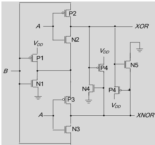
Figure 8. Proposed full swing XOR-XNOR circuit based on GDI Cell.
