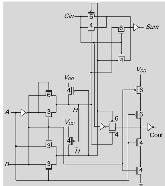
Figure 3. Hybrid-CMOS full adder (Hybrid-CMOS).
