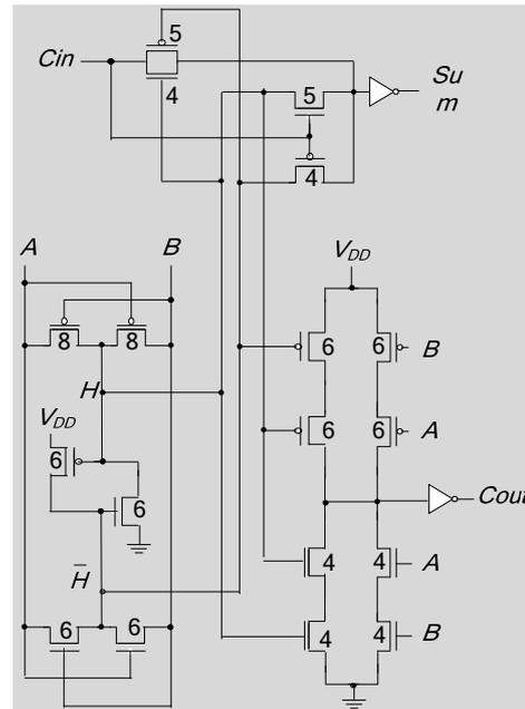
Figure 2. Hybrid pass logic with static CMOS output drive full-adder (HPSC).
