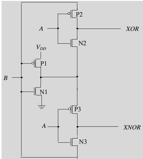
Figure 7. Non-full swing XOR-XNOR circuit based on GDI cell.
