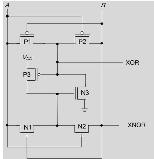
Figure 5. XOR-XNOR based on pass transistor logic in [7].
