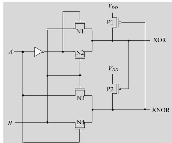
Figure 6. XOR-XNOR based on complementary pass transistor logic in [8].
