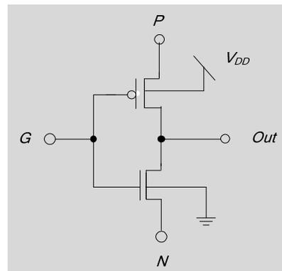
Figure 1. The circuit structure of modified GDI cell.
