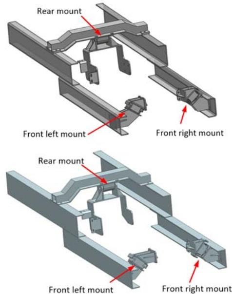
Figure 10. The original design (left) and the new design (right) of the brackets
