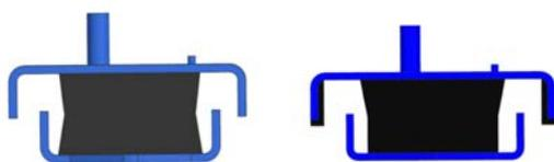
(a) The original design (left) and the new design (right) of the front mount
