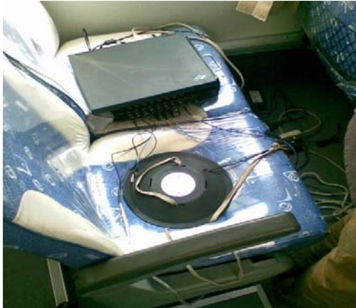
Figure 12. The data collection system and the accelerometer
