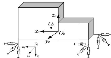
Figure 2. A PMS model and its coordinate systems
