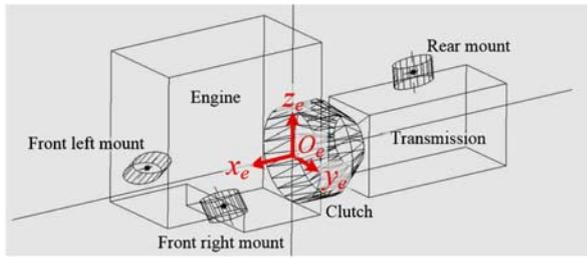
Figure 3. The dynamic model of a PMS
