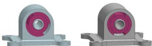
(b) The original design (left) and the new design (right) of the rear mount
