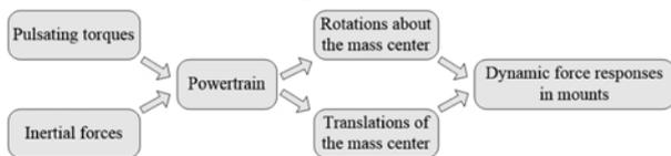
Figure 1. The vibration mechanism of a PMS
