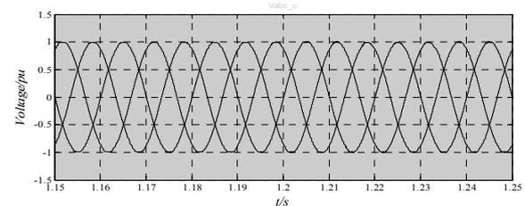
Figure 12. The voltage at the microgrid bus in case 3
