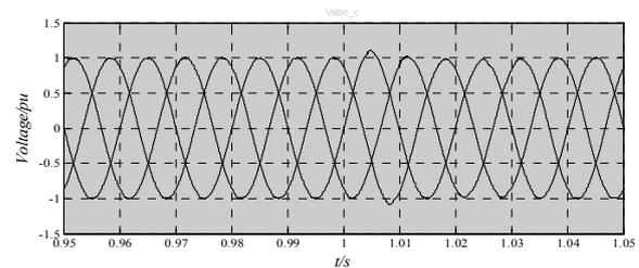
Figure 11. The voltage at the microgrid bus in case 2 at 1.0s
