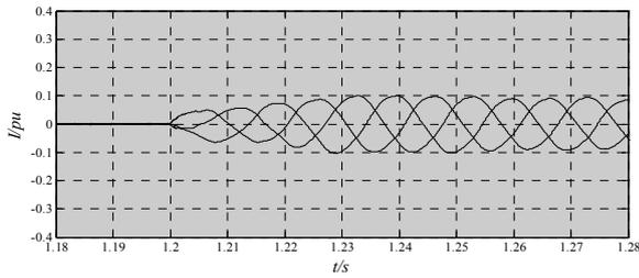
Figure 13. The current of static switch.
