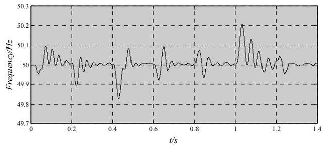
Figure 17. Microgrid voltage frequency
