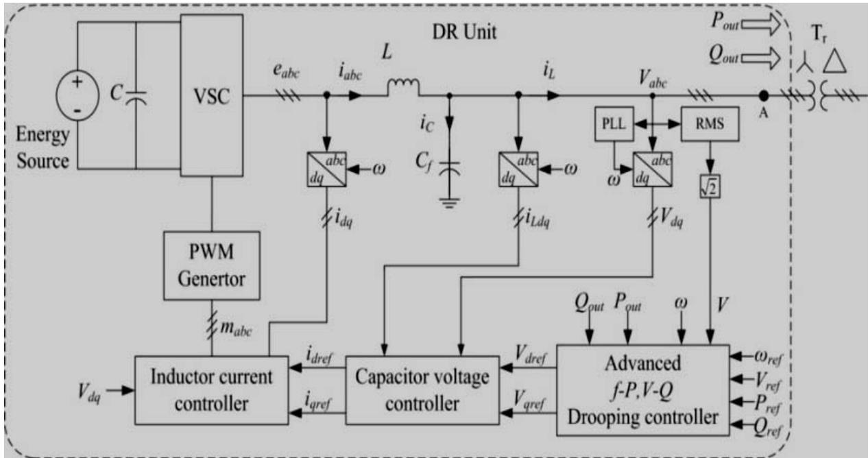
Figure 1. The schematic diagram of the feed-forward f-P/V-Q drooping control method.
