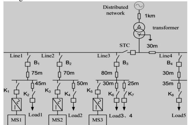
Figure 6. Typical structure of microgrid.
