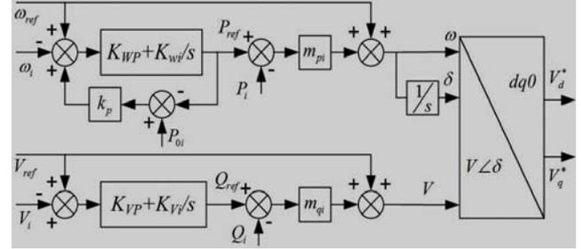
Figure 4. Block diagram of feed-forward f-P/V-Q controller.
