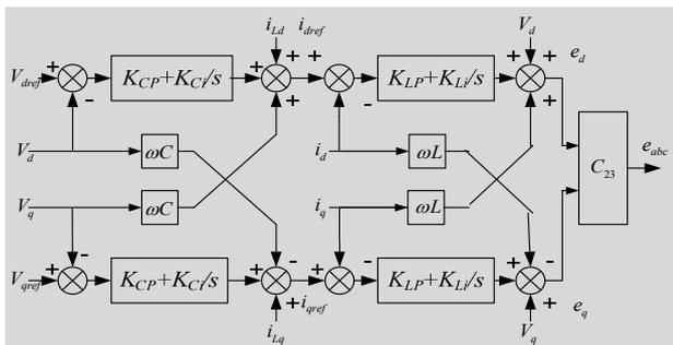
Figure 5. The schematic diagram of capacitor voltage-inductor current controller
