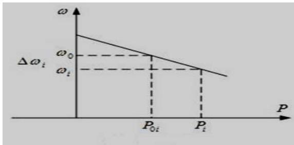
Figure 2. P- $\omega$  Drooping curve
