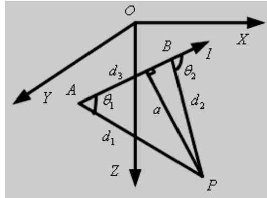
Figure 2. A random linear lead in space with electrical current
