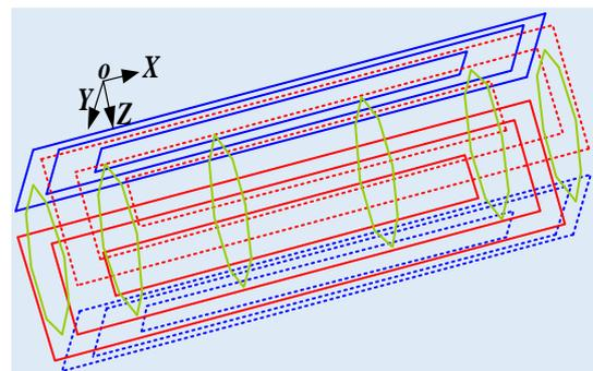
Figure 1. The overall design scheme of the magnetic field generator
