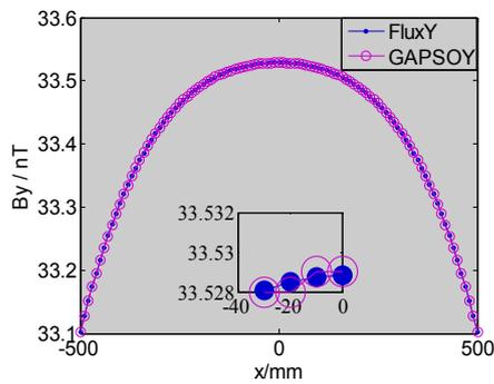
Figure 6. Comparison of  $B_y$  of measured line 2
