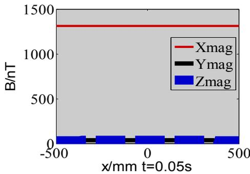
Figure 11.  $B$  simulations results with Flux along measured line
