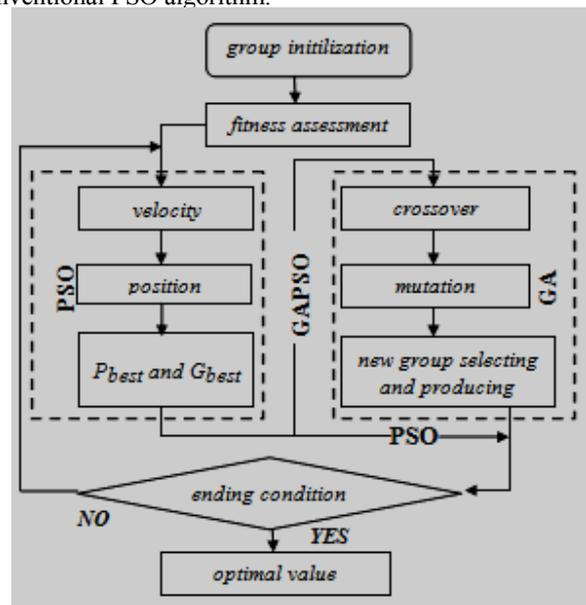
Figure 3. The flow chart of GAPS0 and PSO algorithm
