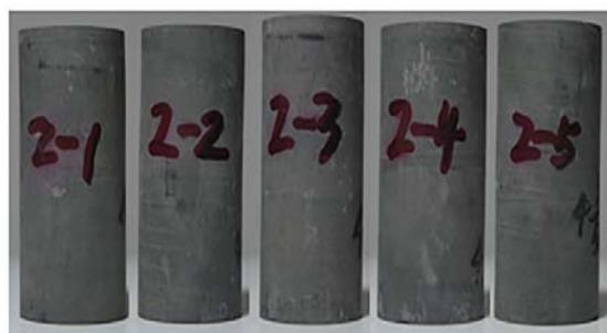
Figure 6. standard cores for triaxial stress test
