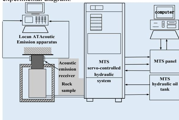
Figure 1. Flow chart of experiments for toughness.
