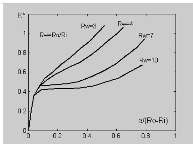
Figure 3. Chart for manual calculation of  $K_{IC}$ .
