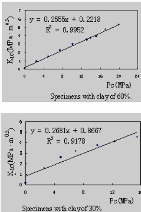
Figure 4. Relationship between toughness and confining pressure.
