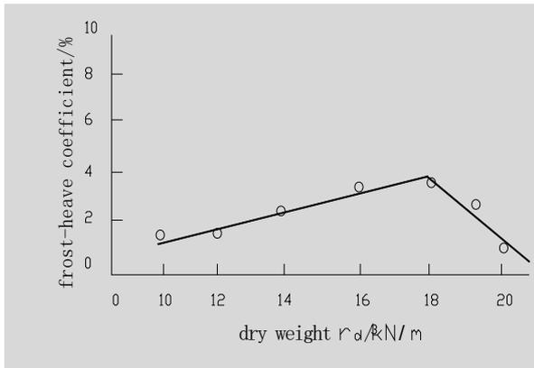
Figure 1. The relationship curve between dry specific weight and its frost-heave coefficient
