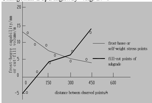
Figure 2. The relationship curve between subgrade cross section forms and self-weight stress with the frost-heave capability
