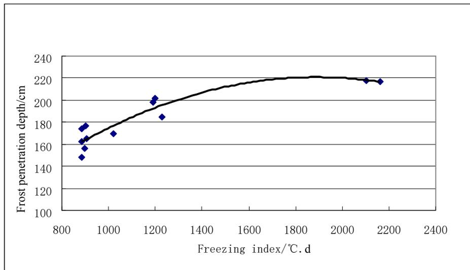
Fig 5 Diagram of frost penetration depth and freezing index
