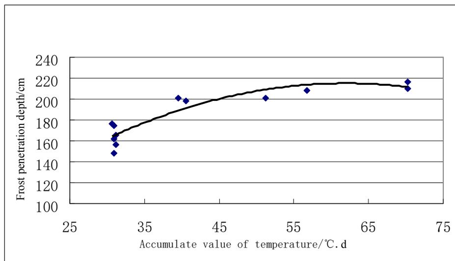
Fig 6 Diagram of frost penetration depth and accumulates value of temperature
