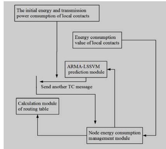
Figure 2. Working principle of EW-OLSR algorithm
