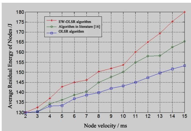
Figure 4. Average residual energy of nodes in different algorithms
