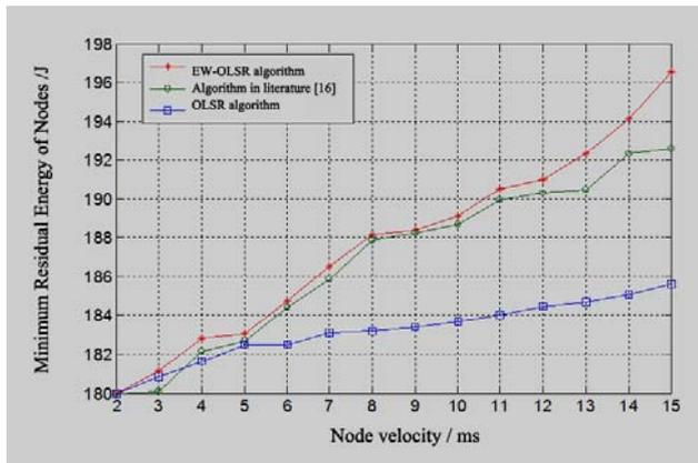
Figure 3. Comparison of minimum residual energy of nodes in different algorithms
