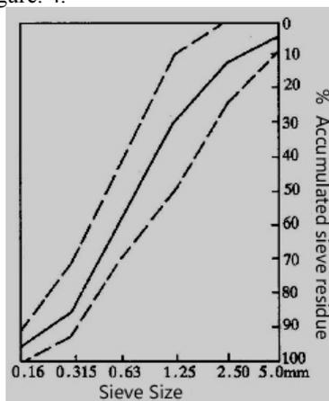
Figure.4 Pump concrete fine aggregate optimum grading chart
