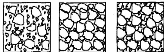
Figure. 1 Suspended compact structure, aggregate framework pore structure and aggregate framework compact structure.
