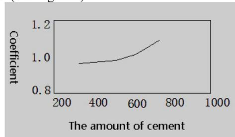
Figure.2. The cement content and concrete shrinkage.
