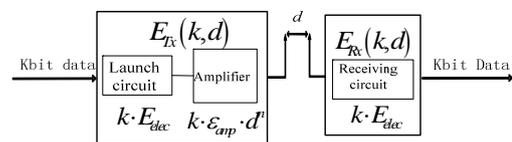
Figure 2. Energy consumption model of sensor node
