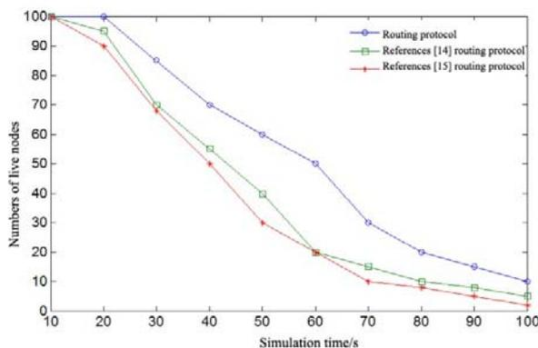
Figure 7. Comparison of network life cycle for different routing protocols
