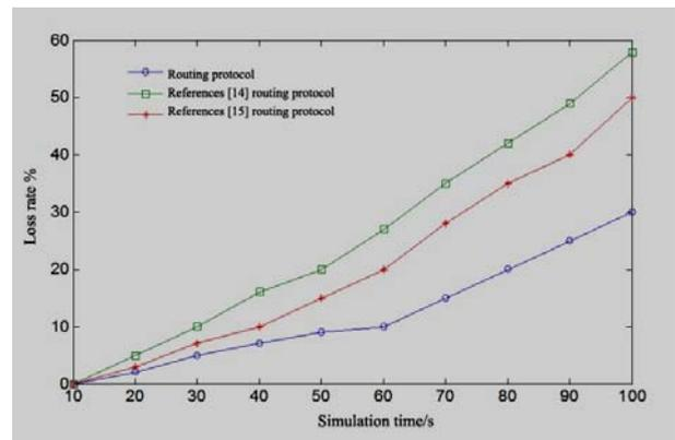
Figure 8. Comparison of packet loss rate for different routing protocols
