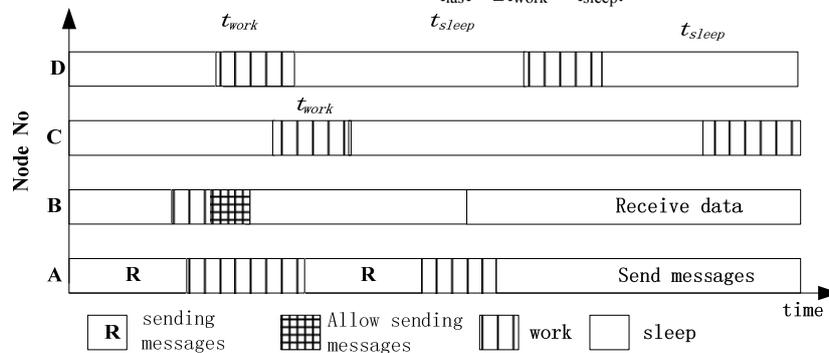
Figure 5. Wake-up procedure of reception of the sensor nodes data
