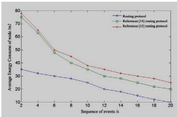
Figure 6. Comparison of average energy consumption of nodes for different routing protocols
